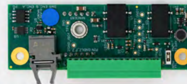
Signal Manager with Master Relay 1200607
